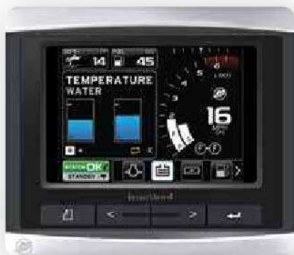
VesselView 4 monitors up to two engines
